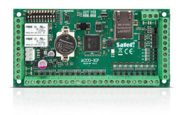
RS-485 bus. In the case of the **ACCO NET** system, the controller connects to the **ACCO-NT** access control panel via the RS-485 bus. In turn, communication between the control panel, the system server and the computer with the **ACCO Soft** configuration program is provided with the use of the TCP/IP protocol.
